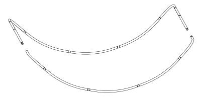
**5.** Connect the top corner tubes #2 on both right and left side of system to the #4 vertical tubes.
