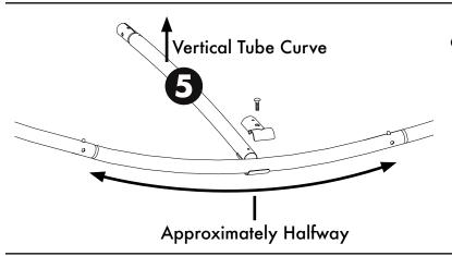
6. With the frame still lying in a "scoop" shape, you will be connecting the clamps. The curve of the vertical tubes will be facing toward the shorter or concave curve of the system. The pins on the vertical center tubes will be facing to the side.
