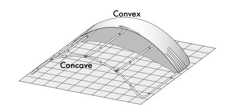
**5.** Stand the frame up and the cover will easily slide down over the frame. Fit the top corners tightly on the frame.
