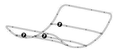
**8.** Next connect the #7 tubes to the #6 tubes. Repeat the step of attaching the clamp portion of the #7 tubes to the top curve at the curve tube midpoints.
