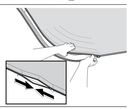
1 1 • When you have finished the zipping and they both meet in the center, move both zipper pulls around to one side to they do not interfere when the structure is standing. Stand the finished structure upright and go around the frame and align the edge seams of the banner with the frame to improve the look of the graphic.
