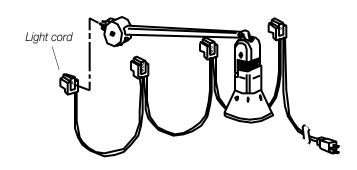
Attach assembled fixture to clip on top section of channel. Hold down locking tab and <u>back</u> fixture into clip.
