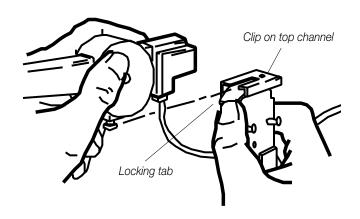
Rotate fixture 90° counter-clockwise.
