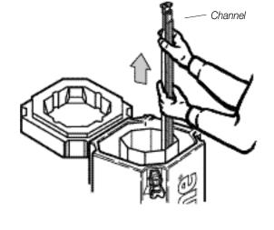
Your channels are hinged for easy set up. The light clip is on the top channel.
