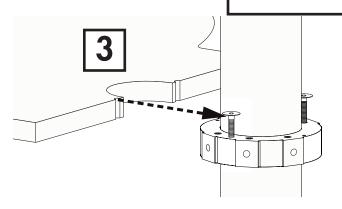
3. Place one half of the counter onto the collar, fitting upper edge of the counter under the heads of the screws The smaller cutouts on the face of the counter will fit against the screws. The screws will hold this half of the counter in place until Step 6.
