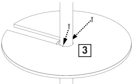
3. Drop the two holding screws into the small holes on either side of the cutout. Carefully rotate the counter top around the tube until the screws drop into the threaded holes in the collar.
